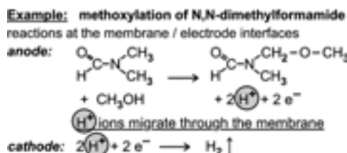
Fig. 2. Scheme of an SPE cell using a cation exchange membrane for the methoxylation of N,N -dimethylformamide [24].
